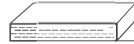
Please note the cutting will expose internal foam structure of the panel. Make sure the cutting edge is at the wall edges and is not exposed.
